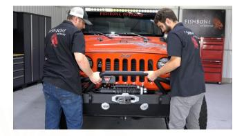
With the help from a second pair of hands, lift the bumper up to the frame of the Jeep and insert the bumper studs into the frame. Using one (1) M10 nut, lock washer, and flat washer per stud, secure the bumper to the Jeep.
