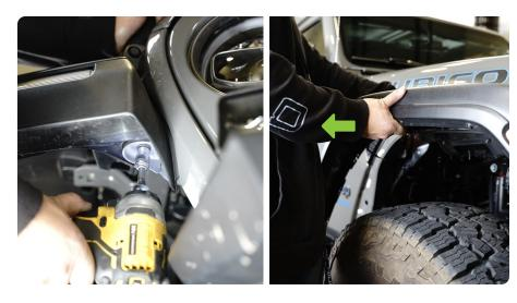
STEP 4 | Use a trim clip tool to remove the factory clips along the fender.
