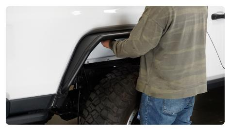
STEP 13 | Install the fender flare onto the vehicle using the provided M8 hardware with a 5mm allen bit (and 13mm wrench if using nuts).
