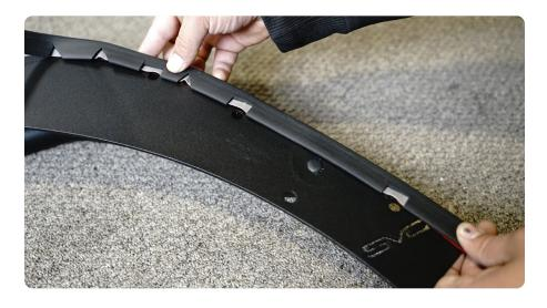
Install the fender flare onto the vehicle using the provided M6x20 hardware with a 4mm allen bit.
