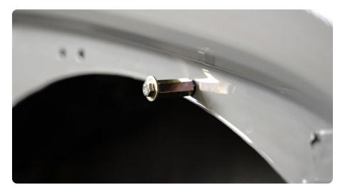
STEP 17 | Use a 12mm wrench to hold the spacer while tightening with a 10mm socket. Tighten slowly until the nutsert is set properly. Do not over tighten.
