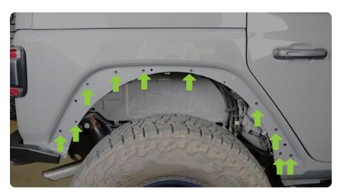
Install the fender flare onto the vehicle using the provided M6 hardware with a 4mm allen bit.
