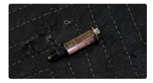
STEP 16 | Slide the nutsert tool with the nutsert into the mounting hole. Ensure the flange of the nutsert is flat against the vehicle prior to tightening.
