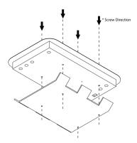
**Step 8:** Secure the mat to the mounted substrate by using the supplied double side mounting pads. Expose one side of the adhesive, and apply to the substrate. Do not block holes for alinement of the rubber mat. Remove the film on the tape and attach the mat. Push the LED through the hole of the mat. Adjust so it is flush to the mat.
