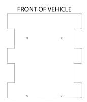
**Step 8:** Place the substrate on the top of the FDMC tray with the LED Hole facing the front of the vehicle. Push the LED into the hole 1/4 past the substrate. Attach to FDMC tray using the following screw options:
