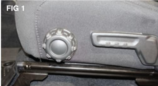
*Put on safety glasses. Open the driver or passenger door of your Jeep. Locate the seat slider. (driver side shown) (FIG1)*
