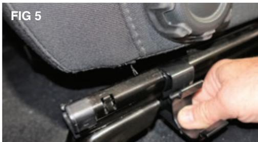
*Tighten the M5 x 45mm Screw until the bracket is snug being careful not to over tighten and damage the bracket. (FIG 5)*
