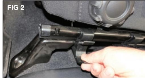
*Snap the light bracket to the seat slider as shown. Slide the front bracket as close to the front of the seat as possible. (FIG 2)*
