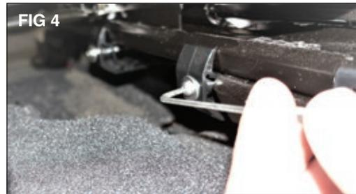
*Using a 3mm Hex Allen Key install one M5 x 45mm Screw and Flat Washer in each bracket. (FIG 4)*
