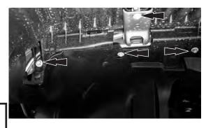
Remove (2) additional factory bolts from inside of splash shield. Save bolts.
