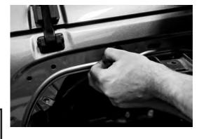
Remove (4) plastic fasteners from the flare and splash shield assembly.
