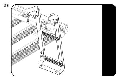
Remove the M8 x 30 Button Head screws from the 2nd and 3rd rear slats, position the assembled ladder onto the side profile and insert the supplied BHM8x30 screws (Item 5) into the 2nd and 3rd slat holes. DO NOT FULLY TIGHTEN.
