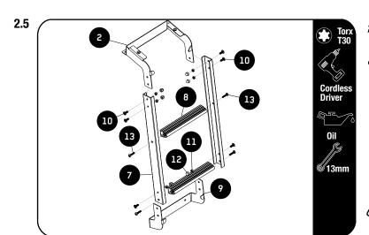
Assemble the Ladder Rung steps (Item 8) to the Ladder sides (Item 7) using the M6 x 25 Thread Forming Screws (Item 13).
