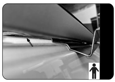
With the help of a friend lift the rear roof slightly to allow the ladder lower bracket to slip in between the roof ledge and the body nanel
