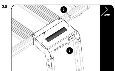
Fit the Top Step Cover (Item 1) and secure using the M6x12 button Head screws (Item 3) fully tighten.
