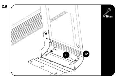
Fully tighten the two bottom M6 Nyloc nuts fitted in 2.7 and place the M6 Nut Caps (Item 12) over the nuts
