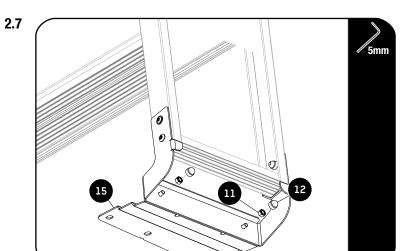
Align the ladder with the Bottom Bracket (Item 15) and thread the M6 Nyloc nuts (Item 11) onto the bottom bracket inserts.
