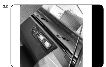
Remove the four screws on the inside rear ledges (2 per side) DO NOT LOOSEN the four smaller screws (2 per side) these are guide pins to re align the roof for fitment.
