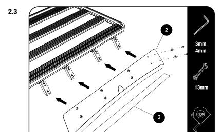
Remove the M5x16 Countersink Screws & M5 Finishing Washers from the bracket.
