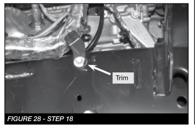
Remove the bracket that attaches the main harness to the frame/coil bucket. Drill a 1/4" hole into the side of the bracket. Then cut the small bent ear off the side. SEE FIGURES 39-30
