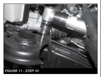
11. Install FT50681 (Driver Coilover Tower) to the factory coil bucket using a supplied 3/8" x 1-1/4" bolt and nut. Then, using a vise grip or clamp. Position the new tower so it is setting flush on the frame then clamp together. **SEE FIGURES 12-13**
