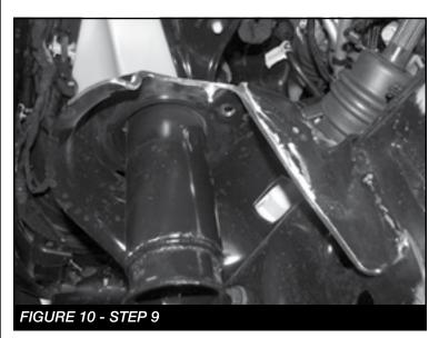
10. Using a drill and 3/8" bit. Drill out the existing hole on the coil bucket. **SEE FIGURE 11**
