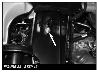
Install FT50692 (Short Nuttab) through the factory hole just left of the new coilover tower using the supplied 1/2-13 x 1-1/4" bolt, flat and split washers. Leave loose. SEE FIGURES 24-25
