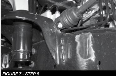
9. Measure 1" from the outside edge of the inner coil bucket lip. Mark a line. Note: Everything past the 1" mark will need to be removed. Using a cut off wheel or saw zaw cut the part off of the bucket. Sand to a smooth finish. Paint all bare areas. SEE FIGURES 8-10
