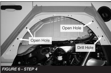
Using a nutsert tool (not included) install the provided four 5/16" nutserts into the holes that were drilled in the last step. SEE FIGURE 7
