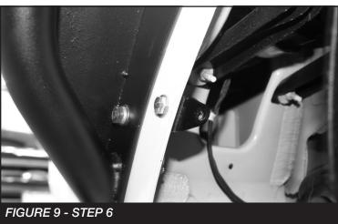
Install the fender inner liner using the factory plastic tabs and supplied tek screws. Cut the liner for proper fit. The screws will be used to mount the inner liner to the tabs installed in the last step. SEE FIGURES 10-11
