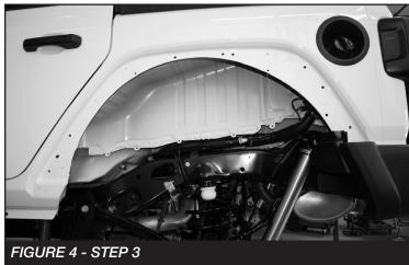
Temporarily install the new fender using two 5/16" bolts and nuts in the center and towards the front. Mark the rear most hole using the fender hole as a guide. SEE FIGURE
