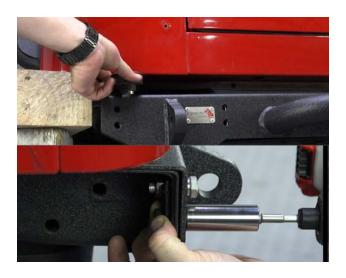
Install the M12 or 7/16" bolts and washers through the bottom of your bumper and into the frame. Compare these with your OEM bolts to check which size is needed for your application.
