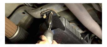
On the rear side of the skid plate, drop the provided 7/16" hex bolt with flat washer down through the top of the crossmember and through hole on the skid plate. Tighten this down with the second washer and nyloc nut using a 5/8" wrench to hold the bolt, and a 5/8" socket to tighten the nut.
