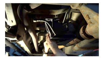
Align the OE canister with your new skid plate to ensure all bolt holes line up. Using your factory hardware, bolt everything in the factory position.
