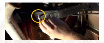
Install your new skid plate using your OE bolts and tighten. Using the supplied M12 washer and locknut, secure the bolt you dropped down through the crossmember.
