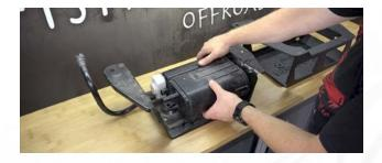
Slip the hardline through the rear of the Fishbone Offroad EVAP canister skid plate. Ensure the mounting tab for the canister is towards the bottom of the skid plate so it can be bolted down.
