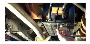
To the right of the electrical connector on the rearmost end of the EVAP canister, remove the upper hardline using two small flat head screw drivers. You will use one screw driver on each side of the c-clip. Each tab must be pried open while simultaneously pulling the clip away. For a visual of this procedure, visit our website and watch our installation video – www.fishboneoffroad.com.
