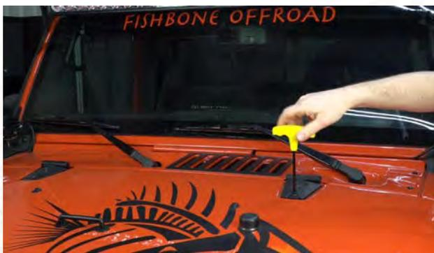
spacers ensuring the mounting hole for the light faces inward towards the middle of the Jeep. Using the supplied bolts, loosely secure the bracket in place. The bracket should be tight enough to keep it from falling over, but loose enough to allow adjustments for the light.
