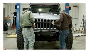
With the help from a second pair of hands, lift the bumper up to the frame of the Jeep and insert the bumper studs into the frame. Using one (1) M10 nut, lock washer, and flat washer per stud, secure the bumper to the Jeep.
