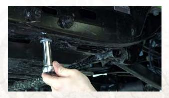
Remove the nuts from the rear-most body mount using a 16mm socket. For 4DR models, repeat this step on the middle body mount.
