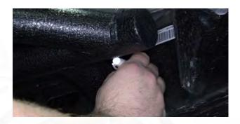
Remove the step slider and drill the marked location with a 7/16" drill bit. Use a smaller drill bit and step up in size if necessary. A centerpunch is also recommended to aid in starting the hole.
