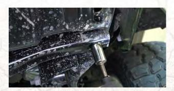
On a 2DR model, it may be required to loosen the skid plate bolt to allow enough flex to fit the new step slider between the frame and crossbar.
