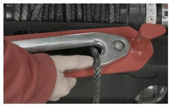
Holding the two parts together, place them up to your bumper and into place using the two included bolts lead by a flat washer.
