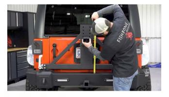
Using the tape measure, measure your wheel offset. Use this number to set the depth of the spare tire bracket. Secure the outer bracket using the remaining two (2) bolts, two (2) washers, and two (2) lock washers.
