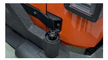
Install your tire carrier stop on the bumper using the supplied M8 hardware.
