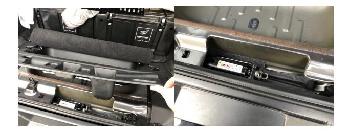
6. Below the factory jack is a drainage plug, remove the plug and make a hole in the plug to insert the wiring harness through. Pull wire through while making sure its secure in the jack compartment. Leave enough lead
