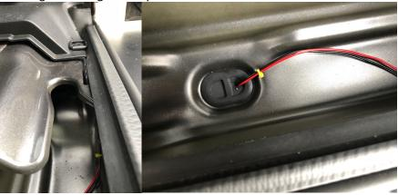
7. Once through the plug, reinstall the plug. Now that the wire is under your vehicle, run your wire securely to your driver's side third brake light under the vehicle. There is a foam insulation panel you will pass through.
