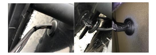
4. You can run the wiring harness through the protective nylon cover that runs from the tailgate to the back inside panel of your jeep if desired. (Or Just zip tie to the protective nylon cover)
