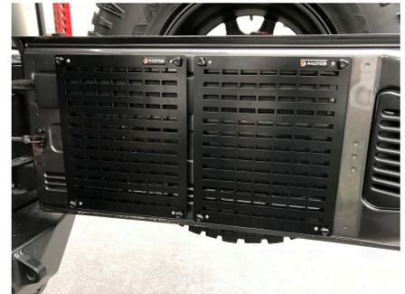
Your GP Trail Tailgate Panel / Table comes with the brackets preinstalled to make installation easier when lining up your panel / table. Installation instructions will be for a single table/ Panel. When installing a second panel for a full kit set up, please repeat steps listed. For lining up the second panel / table, use the first installed panel table for alignment.
