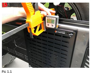
Use a level (Pic 1.1) place on top of your panel to level your panel. NOTE: this will level your panel with the ground. If your tailgate is not level when swung open, you can use the level, but make small adjustments to line up the panel with your tailgate. If you do not want to use a level, just line up your panel and eyeball it to mark your drilling holes. (Pic 1.2)
