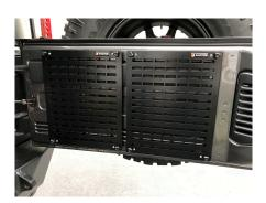
Your GP Trail Tailgate Panel / Table comes with the brackets preinstalled to make installation easier when lining up your panel / table. Installation instructions will be for a single table/ Panel. When installing a second panel for a full kit set up, please repeat steps listed. For lining up the second panel / table, use the first installed panel table for alignment.
