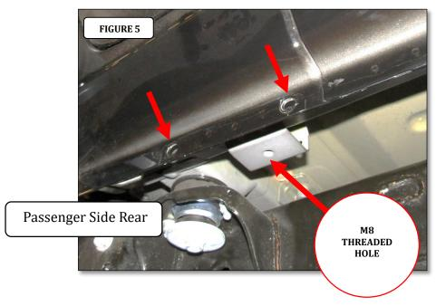
**Step-4** Attach one rear bracket to the pinch mold using (2) 1/4" x 1" hex head bolts, (4) 1/4" flat washers, (2) 1/4" lock washers and (2) 1/4" hex nuts, and to the underside of the body using (1) M8 x 25mm hex bolt, (1) 5/16" lock washer and (1) 5/16" flat washer, (FIGURE 6 & 7). Leave the nuts and bolts loose for final adjustment.
