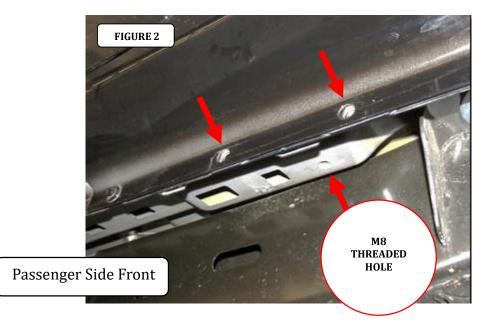
**Step-2** Attach one front brackets to the pinch mold using (2) 1/4" x 1" hex head bolts, (4) 1/4" flat washers, (2) 1/4" lock washers and (2) 1/4" hex nuts, and to the underside of the body using (1) M8 x 25mm hex bolt, (1) 5/16" lock washer and (1) 5/16" flat washer, (FIGURE 3 & 4). Leave the nuts and bolts loose for final adjustment.
