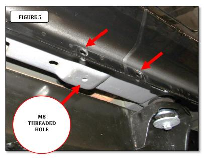
**Step-4** Attach the driver side Center bracket to the pinch mold using (2) 1/4" x 1" hex head bolts, (4) 1/4" flat washers, (2) 1/4" lock washers and (2) 1/4" hex nuts, and to the underside of the body using (1) M8 x 25mm hex bolt, (1) 5/16" lock washer and (1) 5/16" flat washer, (FIGURE 6 & 7). Leave the
