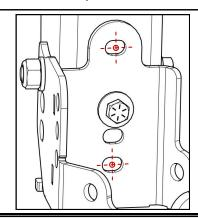
Use a dead blow to bend the front part of the lower skid up and flush against the control arm bracket, as shown.
