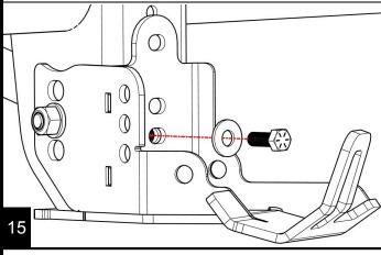
Reinstall the HD skid plate with 3/8" hardware and lightly tighten the bolt.
