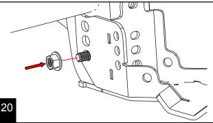
Mark or center punch the second hole down of the back side of the skid plate (see illustration below).
