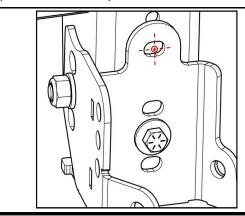
Use a dead blow to bend the front part of the lower skid up and flush against the control arm bracket, as shown.
