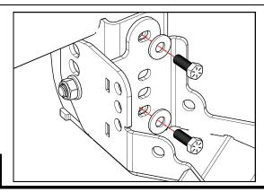
Reinstall the HD skid plate with 3/8" hardware and lightly tighten the bolt.
