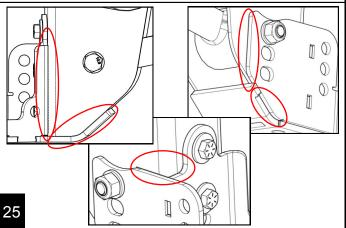
Weld the skid plate to the control arm bracket in location shown below.
