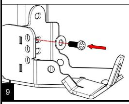
Reinstall the HD skid plate with 3/8" hardware and lightly tighten the bolt.
