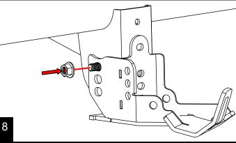
Mark or center punch the top and bottom holes of the back side of the skid plate (see illustration below).
