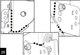
Once welds are cool, paint brackets to protect exposed surfaces. Remove the control arm bolt and reinstall the lower control arm.
