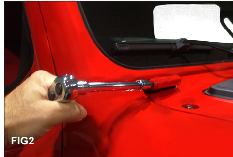
(FIG2) Using a T50 Torx bit socket remove the windshield hinge screw.
