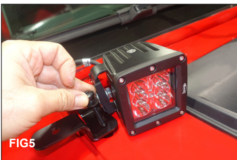
(FIG5) Using a 4mm hex bit driver loosely install the M6 X 1 X 50 Cap Screw and M6 washer.
