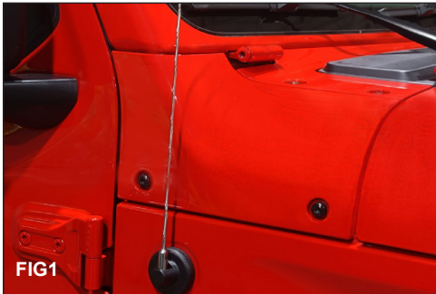
Put on safety glasses. (FIG 1) Using a 3/8" box wrench unscrew the antenna.
