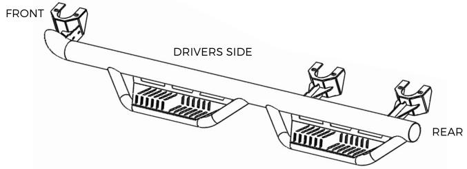
STEP 1: Identify the driver and passenger bars. The tube is cut flat near the rear tire.
