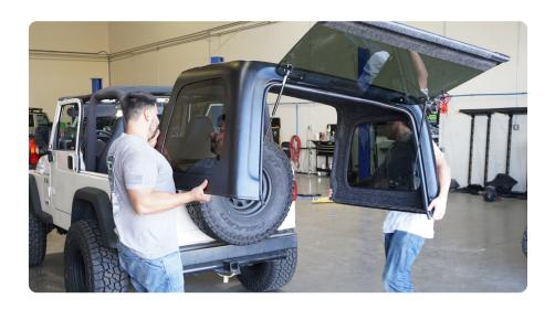
STEP 10 | Adjust the hardtop forward as much as possible so it is sitting flush with the body of the jeep in the rear.
