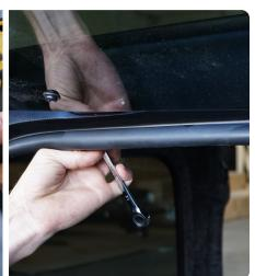
STEP 8 | With the window secured to the top, carefully lift the back window and install both struts onto the hardtop by pressing firmly.
