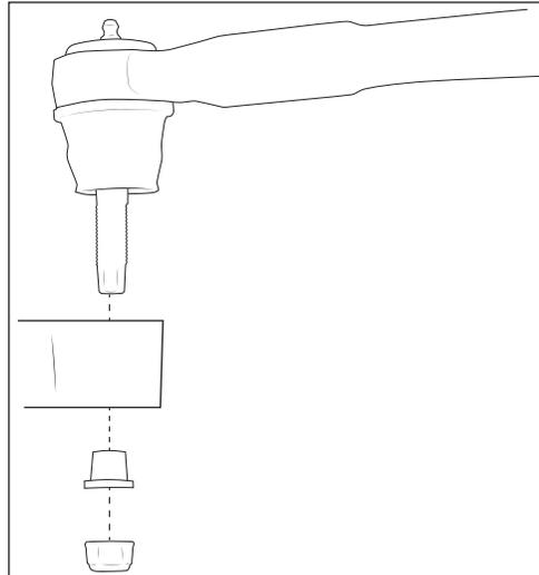
5. Grease draglink socket through the zerk until grease purges around the boot seal; wipe off excess grease.
