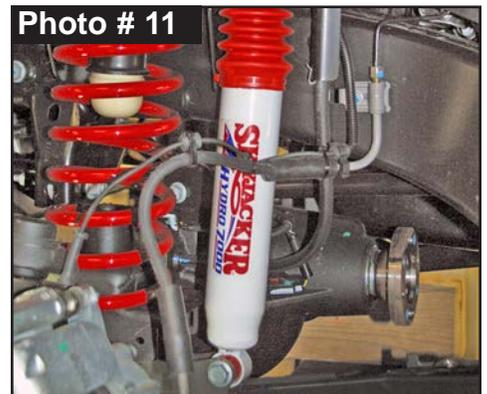
19. Install Skyjacker ADX front shock. **Tech Note:** ADX Remote Reservoir are to be mounted with the remote reservoir toward rear for proper clearance (opposite side of coil spring mount). (See Photo # 12 & # 13)
