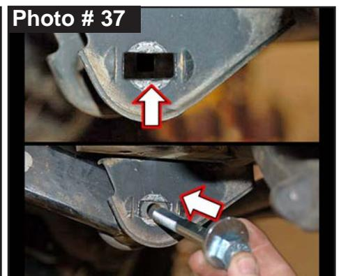
3. Connect OEM front lower control arm to modified OEM front axle mount using Skyjacker eccentric cam bolt, eccentric washer, nut, a 21mm socket \ wrench & a 24mm socket \ wrench. (See Photo # 38)
