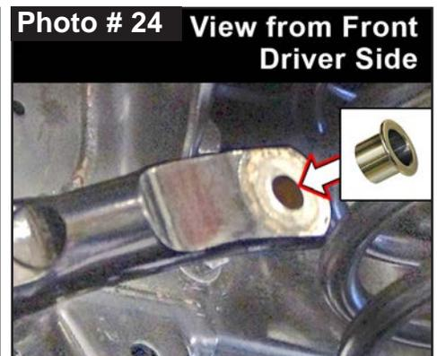
23. **Note:** Skyjacker # 1412BSG-S Sway Bar Reducer Bushing is supplied for **All 2024+ Models**.
