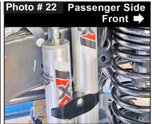
Locate Skyjacker ADX front shock. Loosely assemble two (2) supplied reservoir clamps with two (2) supplied
