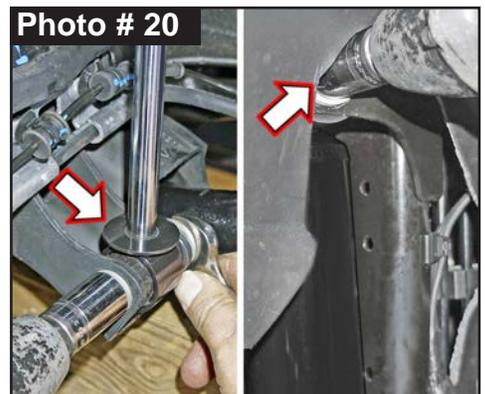
Connect Skyjacker shock at lower axle mount with OEM hardware using a 18mm socket \wrench. (Photo # 20) Secure,
