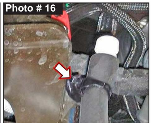
17. While checking for appropriate slack in ABS lines, brake lines, axle vent hose & etc. Lower front axle. Remove OEM front coil springs & rubber isolators.
