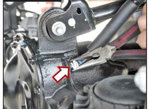
28. **Rubicon Models:** Connect OEM front locker on driver side.
