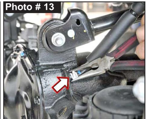
15. Disconnect OEM vent hose \ clip from front differential using pliers. (Photo # 13)
