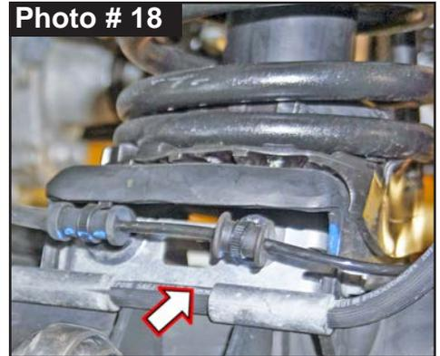
Reach under spring mount pad & above axle tube to install supplied 3/8" SAE Washer & 3/8" Nylon Insert Lock Nut onto bolt. Tighten bump stop spacer into place
