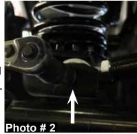
8. Tighten the supplied jam nut of the new Skyjacker adjustable front track bar using a 1 1/8" wrench.
