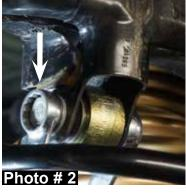
8. Tighten the supplied jam nut of the new Skyjacker adjustable rear track bar using a 1 1/8" wrench.
