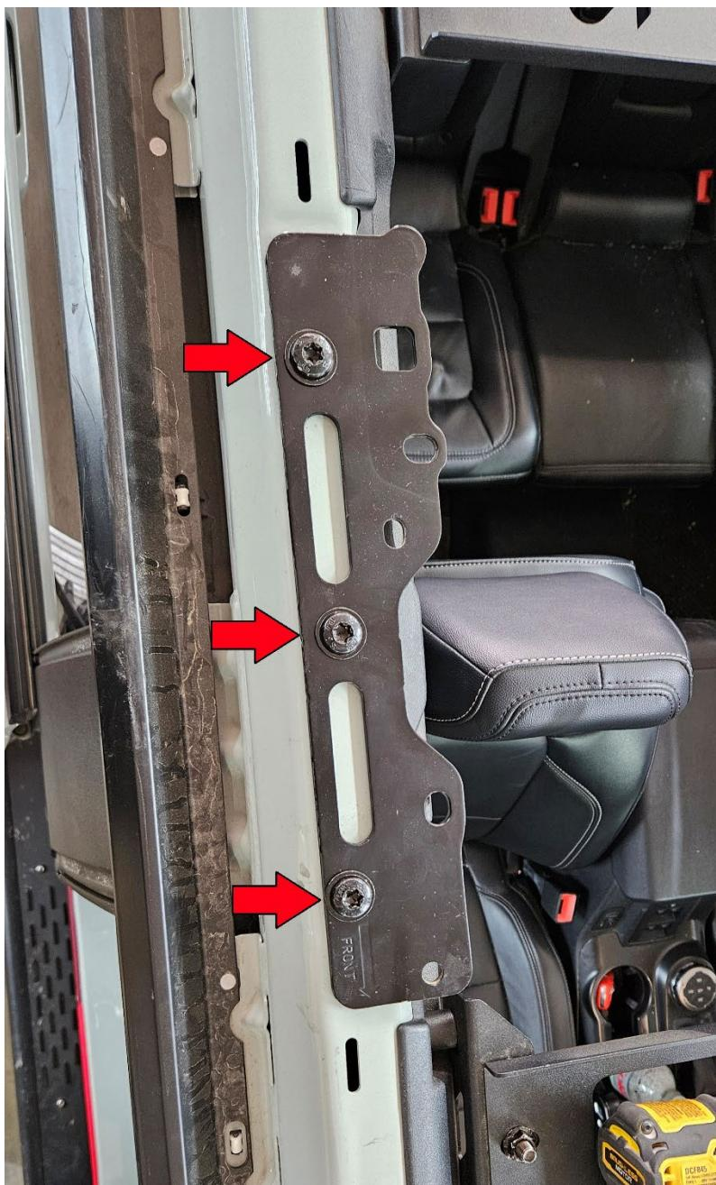
**Step 3:** Place Turn Offroad Bronco Cage Brace on the vehicle and align with mounting holes.
