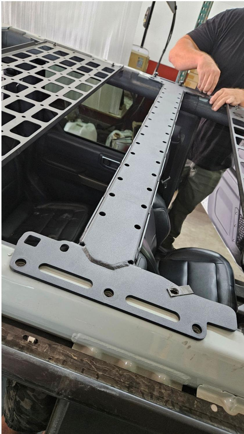
**Step 4:** Install hardware. Insert the M8 hardware provided, starting all 6 fasteners before tightening. To avoid the possibility of fasteners losing, ensure that all fasteners have lock washers and flat washers as shown.
