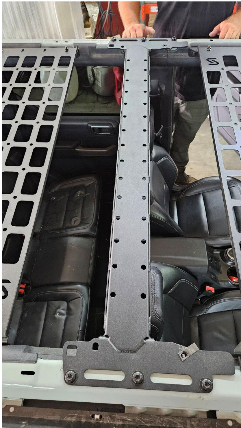
**Step 6:** If using the Turn Offroad Hardtop ensure nut clips are installed on your new cage brace.
