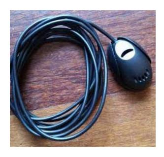
This external mic will work at just about any location, but we do have some recommendations as to placement. Try to keep this mic away from any windows, air vents, or speakers to avoid background sounds or feedback. The external mic will plug into the back of the TJ1002 via a 3.5mm headphone jack plug located just to the left of the RCA pigtail.
