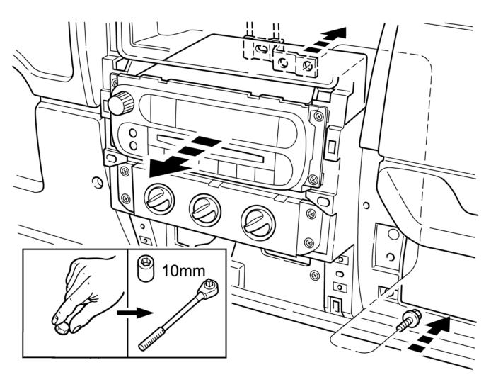
Once the security bracket is disconnected, you can remove the four screws on the faceplate of the old stereo and the whole thing will slide out. Disconnect the antenna and the old wiring harness from the factory harness.
