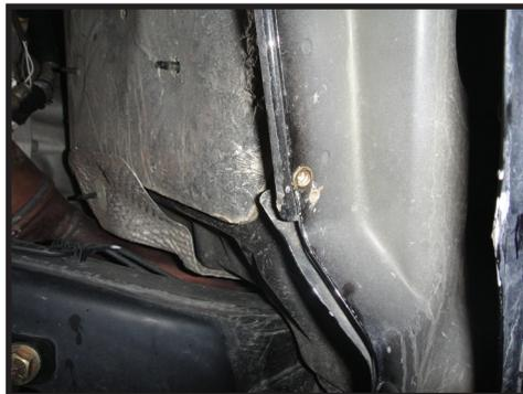
**10.** Mount/hang the fender liner using the factory screws, but leave loose. Use the supplied 10-32 screws and a 1/8" Allen to fasten the fender liner to the rivet nuts on the fender. [Torque to 25 in-lbs]. Tighten factory bolts to factory spec using a 10mm. [FIGURE 9]
