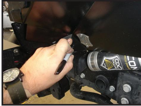
**4.** Mark the hole location of the front vertical portion of the fender liner on the fender sheet metal. [FIGURE 5]
