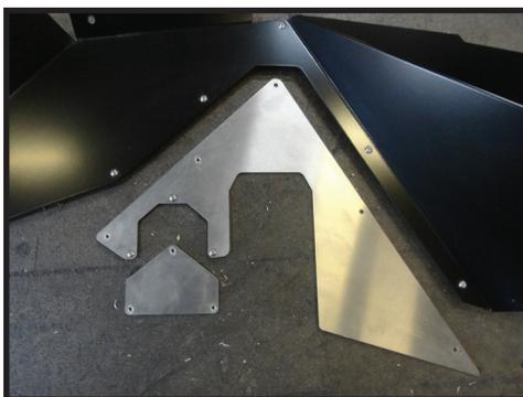
**2.** With factory fender liner removed, use the (2) factory screws and a 10mm to mount/hang the fender liner to the top of the fender. Tighten slightly. (Refer to Figure 2) Make sure the front vertical portion of the fender liner is on the outside of the fender and flush against it. [FIGURE 2 & 3]
