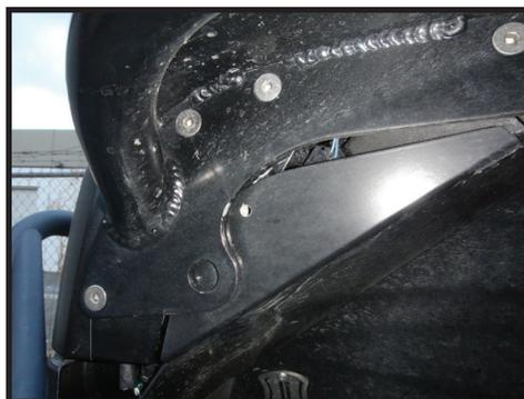
**3.** Hold the front of the fender liner against the sheet metal of the fender body mount. Mark the hole location, transferring it from the hole in the fender liner. [FIGURE 4]
