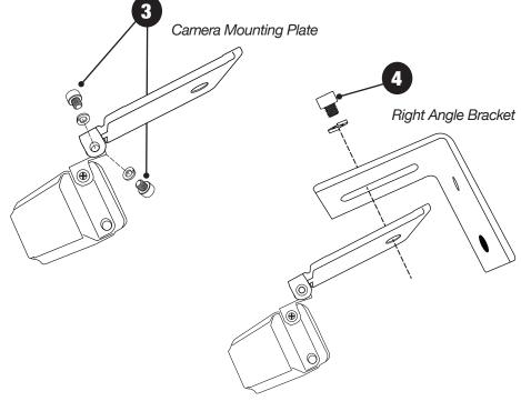
5A. For most appliacations with stock/standard wheels, attach the camera bracket assembly to the Wheel Bracket using a M6 x 1 screw and lock washer.
