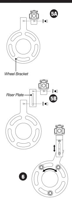
Once positioned, tighten all camera bracket hardware and lug nuts.
