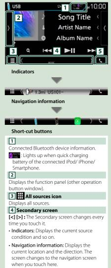
Short-cut buttons: The source changes to the one you have set as a short-cut. For the short-cut setting, refer to <u>Customizing</u> <u>Short-cut buttons on HOME screen</u> (P.17).
