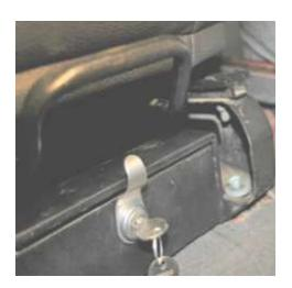
With both front bolts removed slide the drawer unit under seat base so that the tabs with slots of the drawer are under the driver seat front, then replace the two 8mm bolts removed earlier. Tighten the bolts making sure the bolts are down through the driver seat base and through the slots of the drawer unit.
