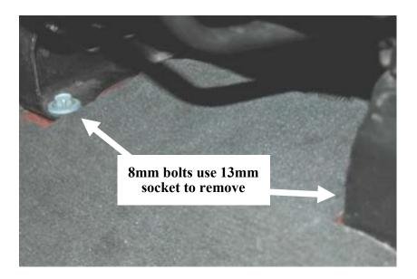
Slide drivers seat back to access the front seat bolts. Remove the front bolts with a 13mm socket on ratchet.
