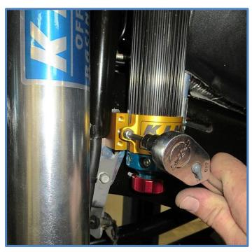
11. Place the rod end into the lower mount, install the factory bolt and tighten to 60 ft-lbs.
