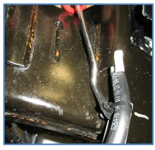
5. <u>Installing reservoir brackets</u> – First bolt the clamp to the reservoir bracket using the provided 1/4 X 1" FHCS (CB5501) using a 5/32 Allen wrench. Be aware the brackets are side specific. Photos show the RIGHT SIDE. See below for proper orientation.
