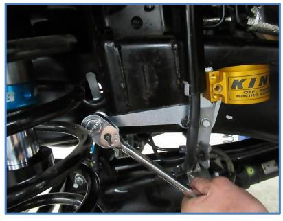
9. <u>Installing Shocks</u> – Be aware the shocks are side specific, make sure you have the proper shock for the side you are working on (photos below show LEFT SIDE). Begin placing the shock into position on the vehicle while inserting the reservoir into the clamp. Place the end cap into the upper mount, install the factory bolt and tighten to 60 ft-lbs.
