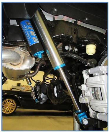
**DOUBLE CHECK ALL HARDWARE:** Make sure everything is installed correctly and all hardware is tight before reinstalling tires. Install tires; remove jack stands and lower vehicle to the ground. Recheck all hardware and lug nuts after 100 miles and periodically after that as part of routine maintenance.
