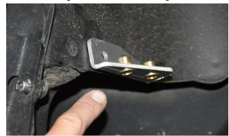
**20. Use the remaining hole in** the bracket as your drill guide to drill a 5/16" hole through the wheel well sheet metal. While drilling, be mindful that the bracket doesn't move and allow the bit to "walk". Be careful as the drill bit breaks through, that it doesn't catch and deform the hole.
