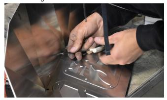
28. Install the supplied Edge Trim along the edge of the Inner Fender Arch. There is a pre-applied adhesive inside the crease of the edge trim.
