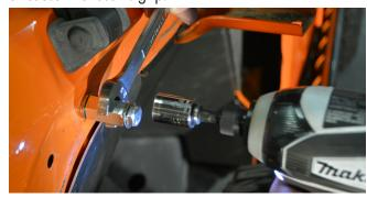
5. Once the nut-sert has seated correctly, loosen the bolt then remove it and the rest of the tool from the nut-sert. Install a new nut-sert onto the tool, oriented the same as the last, and set it aside until your next nut-sert installation. Inspect the nut-sert to make sure it is properly seated and that the surrounding sheet metal isn't excessively deformed. Note that some deformation of the sheet metal is normal, and that it will be covered by the part after installation.
