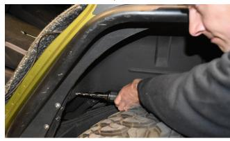
**10. Install a 1/4-20 nut-sert into** each of the three holes just drilled out to 25/64". Again, we recommend the use of a professional nut-sert installation tool.
