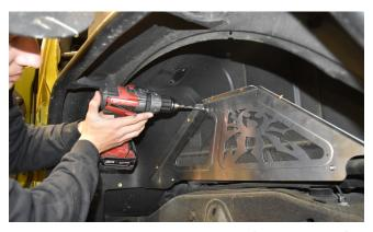
13. Remove the two SS Button Head Cap Screws that had temporarily held the Inner Fender Panel in place, and remove the Inner Fender Panel.
