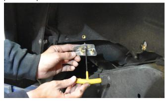
19. Tighten the Button Head Cap Screw while making sure that the bottom edge of the bracket stays parallel with the bottom edge of the wheel well sheet metal. Make sure the fastener is tight and the bracket is snug.
