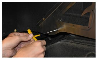
**12.** Use the installed Panel as a drill guide to drill 5/16" holes into Jeep's wheel tub sheet metal, at locations denoted by the two holes at the top of the Panel.
