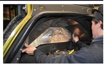
**30.** Install the supplied 1/4-20 X 3/4 SS Button Head Cap Screws at each of the four hole locations in the Inner Fender Panel. There are two along the top and two along the bottom. Leave them slightly loose.
