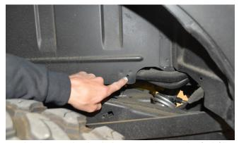
On the driver side, this hole is very close to the fuel filler hose. When drilling, be very careful to not contact or puncture the fuel filler hose, especially when the drill bit "breaks through", and the pressure you are applying to the drill motor may cause the bit to slip suddenly forward. To prevent this, decrease pressure before the bit finally breaks through.
