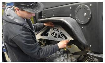
**14. Drill the two new holes** (that were pilot-drilled in the previous steps) out to 25/64". Again, be careful to reduce pressure before the bit breaks through, to avoid damage to interior coverings.
