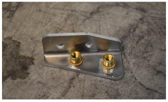
**18. Install the JK Rear Inner** Fender Front Bracket - Left into the front wall of the driver side wheel well. Start by using one of the supplied 1/4-20 X 3/4 SS Button Head Cap Screws, through the right-side hole (see the photo below) into the 1/4-20 nut-sert that was installed in a previous step.
