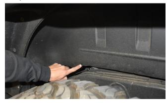
8. The third existing hole to be drilled out is located along the lower edge of the forward wall of the wheel well, as shown:
