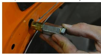
4. Use an open end wrench to hold the coupler nut stationary while turning the head of the bolt clockwise with a ratchet (or small impact wrench) and socket. As you turn the ratchet, the bolt will draw the far end of the nut-sert toward the inside of the sheet metal, gripping it with the knurled outside edge of the nut-sert as it deforms. Continue to turn the ratchet until the nut-sert is fully seated. DO NOT OVER-TIGHTEN as you can damage the nut-sert, or cause it to lose its grip.
