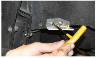
**24. Install the JK Rear Inner** Fender Fill Plates (-Front and -Rear) into the JK Rear Inner Fender Panel. They will fit into the slight depressions formed by the bead-rolled feature, on the back-side of the Inner Fender Panel.
