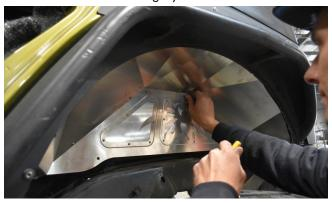
**31. Install the supplied 1/4-20 X** 3/4 SS Button Head Cap Screws into the two locations at the bottom of the forward panel of the Inner Fender Arch.
