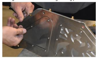
**26.** Attach the JK Inner Fender Arch - Left to the JK Inner Fender Panel - Left. Note that the - Left (driver's side) pieces have corresponding cut-outs where they meet toward the rear of the assembly (see photo below), to clear the fuel filler hose on the Jeep. The Arch piece should be set to the inside of the bolt flanges on the Inner Fender Panel, as shown in the photo below.
