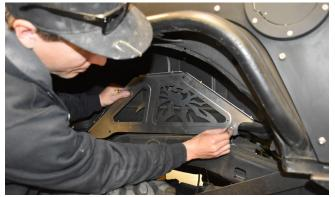
Use the supplied 1/4-20 SS Button Head Cap Screws at these two locations to hold the panel firmly in place.
