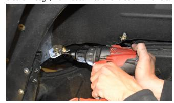
**21. Loosen the single Button Head** Cap Screw, and swing the bracket down and out of the way, allowing access to the hole that was just drilled through the wheel
