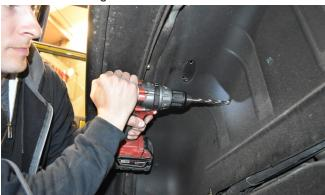
**15. Install a 1/4-20 nut-sert into** each of the two new holes just drilled out to 25/64". Again, we recommend the use of a professional nut-sert installation tool.
