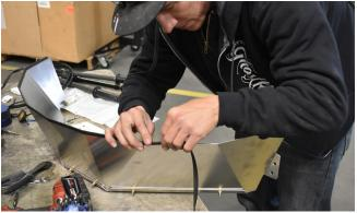
Press the edge trim firmly onto the edge of the sheet metal in order to properly seat it as well as activate the adhesive. Trim the Edge Trim as needed.
