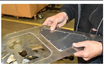
25. Use the supplied #6/32 X 1/2 SS Button Head Cap Screws to attach the Fill Plates. Orient the fasteners with the screw heads to the outside of the Inner Fender Panel (as shown in the photo below) with a supplied #6 SS Flat Washer and #6-32 Nylon Insert Lock Nut on the back side. Leave each fastener loose until they are all installed, then tighten them in an alternating crossing pattern.
