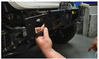
Note that the Spacer Plates are not symmetrical and must be oriented correctly, to match the four corresponding bolt holes in the Cradle and the frame. The space between the bolt holes and the edge of the spacers is wider along one edge. The Spacer Plate should be oriented so the edge with the wide space is at the top, as shown in the photo above. A spud bar or pry bar will be helpful in fine-tuning the placement of the spacer plate.
