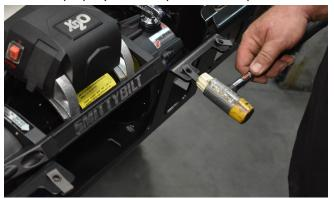
17. Pre-position the two Frame Mount Spacer Plates, between the Recessed Winch Cradle and the bumper mounting flanges on the ends of the Jeep's frame rails. Slightly loosen the fasteners for the previously-installed Winch Cradle Brackets, if necessary, to allow necessary movement of the Cradle. But keep the fasteners tight enough to hold the Spacer Plates in place, once positioned.
