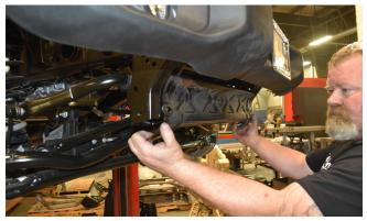
**4.** If your Jeep is equipped with factory fog lamps, reach behind the bumper and disconnect the fog lamp wiring harness from the chassis wiring harness.
