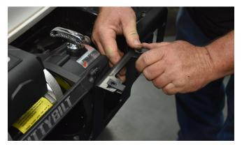
**16. A rubber mallet or soft** dead-blow hammer may be needed to properly seat and position the clip-nuts.
