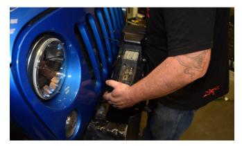
**13. Install the four mounting bolts** that came with your winch, through the bottom of the Recessed Winch Cradle, into the mounting nuts in the winch.
