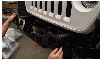
**9. Use the stock bumper bolts** to install the Winch Cradle Mounting Brackets on either side of the Winch Cradle, to fasten it to the inner frame rails.
