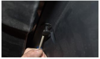
With the fasteners removed, remove the plastic lower air dam and set it aside.
