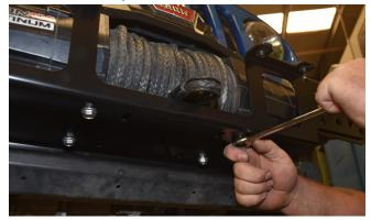
**15. Install the supplied 5/16-18 clip-nuts** into the four nut flanges along the front of the Recessed Winch Cradle. Make sure that the extruded barrel of the clip-nut points downward through the hole in the flange.
