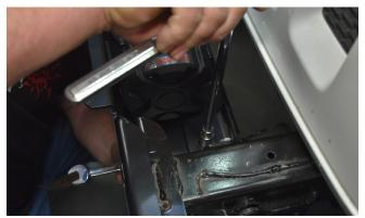
12. Place the winch into the Recessed Winch Cradle. If the winch is new, install it without the cable or rope. If the cable or rope is already installed, it will need to have a removable hook or thimble. Otherwise the cable or rope will need to be un-spooled prior to this step, and respooled after the end of the bumper installation. It is also recommended to hook up your winch wiring at this time.
