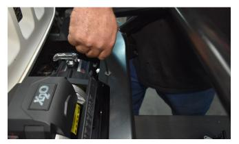
Use a wrench to final-tighten the flat head cap screws. Note that stainless steel is a softer alloy than the hardened steel of the clip-nut, and it may gall or strip if crossthreaded or over-tightened. Do not over-tighten.
