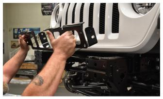
Temporarily "hang" the Cradle by the resting the rightangle flanges on to the tops of the Jeep's bumper mounting flanges.
