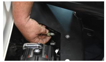
The best strategy is to first try to get one nut threaded on, on either side of the bumper, to start. Once there is at least one nut started on either side, it will be easier to coax the remaining threaded studs through their corresponding bolt holes.
