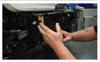
A piece of packing or masking tape might be helpful to hold the spacer plate in place until the bumper shell is installed.
