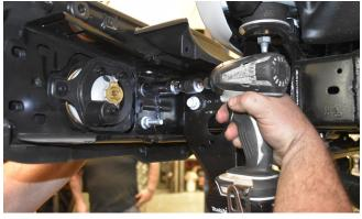
With these nuts removed, remove the bumper from the Jeep.
