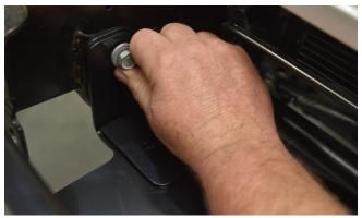
Note that the Winch Cradle Mounting Brackets are specific for the left and right side. They slip on to the Winch Cradle as shown, so that they sit above the bottom surface and outboard of the side flanges of the Winch Cradle. (photos shown without the Winch Cradle installed onto the Jeep, for clarity)
