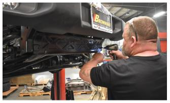
with the bolts removed, slide the metal air dam retainer bracket upward to slide the upper tabs out of the frame horns.
