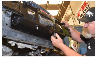
**14. Tighten the four winch bolts** to whatever specification is recommended by the winch manufacturer.
