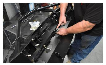
**20. With the help of a** friend, move the bumper (and preinstalled skid, if desired) into position close to the front of the Jeep. A padded surface to set the bumper close to the Jeep is helpful. Thread the end of the winch rope (if present) through the fairlead. Also make sure the wiring pigtails for the LED lights are positioned out of the way, so they don't get caught between bumper mounting surfaces.
