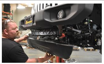
3. Un-bolt the metal air dam retainer bracket.
