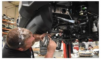
Use a push-in retainer removal tool to pop out the plastic push-in retainers along the front edge of the air dam. If you do not have a push-in retainer tool, a flat-edge screwdriver or small pry-bar may be used.
