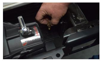
**11. Semi-tighten all hardware for the** Winch Cradle Brackets. Do noght fully tighten these fasteners at this time, as some slight adjustments may be necessary.
