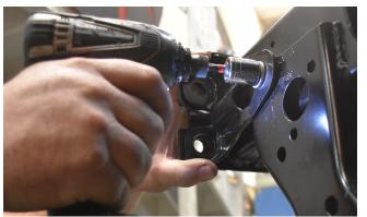
**8. Drop the Recessed Winch Cradle** into place between the frame rails.
