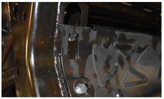
Remove the metal air dam retainer bracket and set it aside.
