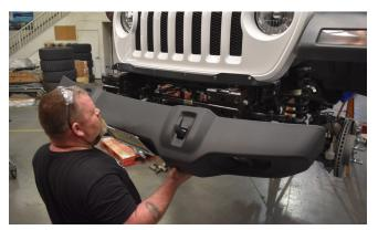
**7. Remove the bumper retaining bracket** from the side of the frame rail.
