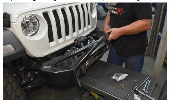
**21. There are floating bolt plates** pre-installed inside the Bruiser bumper. These bolts interface with the four large bolt holes on each of the two mounting flanges on the ends of the Jeep's frame rails. The bolt plates are "floating", that is, they can move around slightly, in order to accomodate slight variations in the Jeep manufacturing tolerances. However, this can make it somewhat tedious to get all 8 mounting bolts started into their corresponding bolt holes.
