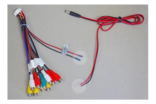
Protect the head unit by ensuring that the electrical connection is safely insulated.
