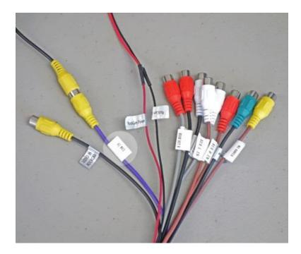
Next, you must connect the "Reverse Trigger" wire on the main harness to a wire in your dash that provides +12V when the vehicle is in reverse. If no such signal is present in your dash, you can extend a wire to your reverse light circuit.
