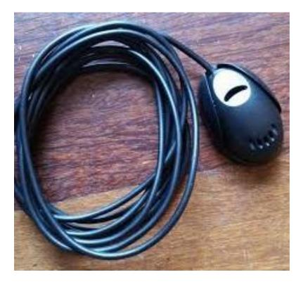
This external mic will work at just about any location, but we do have some recommendations as to placement. Try to keep this mic away from any windows, air vents, or speakers to avoid background sounds or feedback. The external mic will plug into the back of the DD2001 via a 3.5mm headphone jack plug located next to the AM/FM antenna port. Most folks do well placing this directly on the steering column as far away from your gauge cluster as possible.
