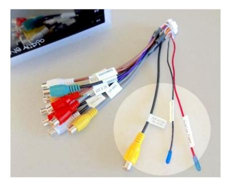
Before making any connections, unplug the A/V pigtail from the head unit and make sure that everything is powered off.
