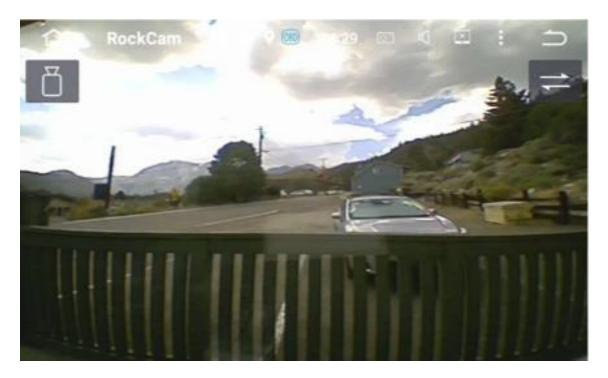
If you see a "No signal" warning, ensure that the front video feed is connected to "RockCam Video In" RCA port and the power wires are properly connected.
