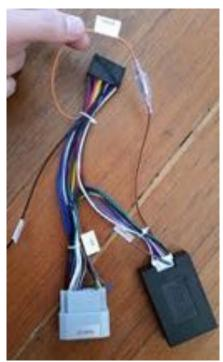
When this wire is connected, your JK2001 will automatically display the backup camera anytime the vehicle is in reverse.
