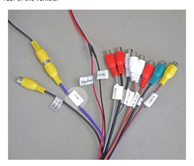
Next, you must connect the backup trigger wire, labelled "REVERSE" on the main wiring harness. This triggers the JK2001 to immediately display the feed from the camera, when the vehicle is backing up.
