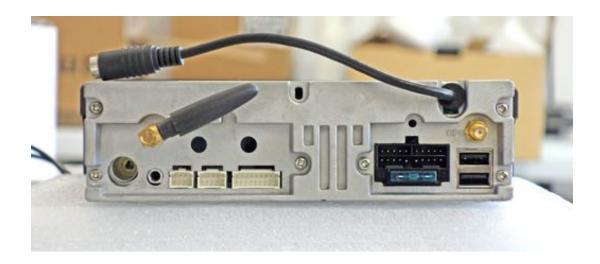
Your Wi-Fi antenna will screw on as shown above. Along with that, your GPS plug in is now on the far right hand side of the JK2001.
