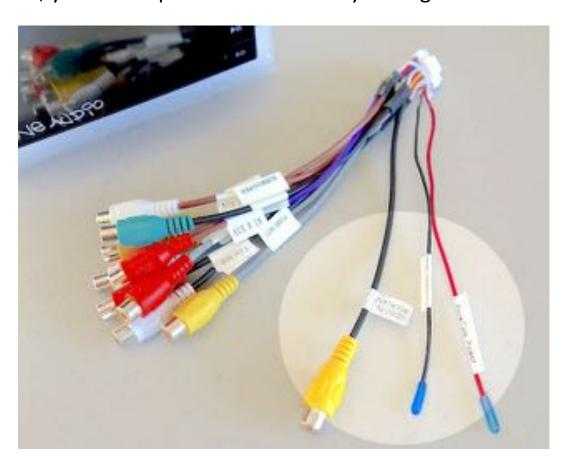
Before making any connections, unplug the A/V pigtail from the head unit and make sure that everything is powered off.
