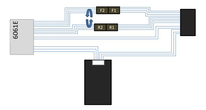
If your vehicle is not equipped with the OEM Alpine Premium Sound System or if you are using your own aftermarket amps and speakers you do not have to make any changes. F2 should be connected to F1 and R2 should be connected to R1 as shown above.
