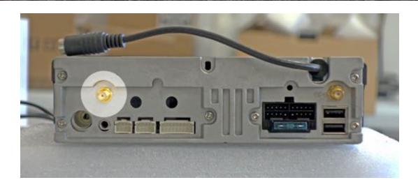
Above is a picture of the back of your JK2001. Your JK2001 is equipped with a Wi-Fi antenna, and you will have this gold plated plug just above the microphone plug in.
