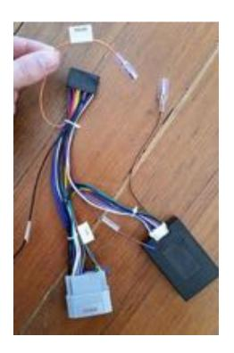
Disengaging this wire will disable a "no signal" warning every time you put your Jeep into reverse when no camera is detected. You can always re-connect this wire when you are ready to install a backup camera.
