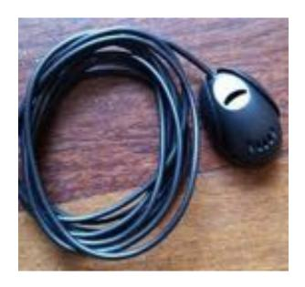
This external mic will work at just about any location, but we do have some recommendations as to placement. Try to keep this mic away from any windows, air vents, or speakers to avoid background sounds or feedback. The external mic will plug into the back of the JK2001 via a 3.5mm headphone jack plug located just to the left of the RCA pigtail. Most folks place this directly on the steering column.
