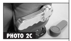
**2.** Your new billet handle has a set screw in the backside of the handle. Align the handle back onto the factory post (See Photo 2A) and tighten using a 1/16" allen key (See Photo 2B). Repeat for the other side and you're finished (See Photo 2C).
