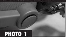
**1.** Begin by removing the factory plastic cover located in the center of the seat handle.
