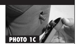
**1.** Begin by using a set of needle nosed pliers to locate and remove the retaining clip behind the seat handle (See Photo 1A & 1B). Remove the factory handle (1C).
