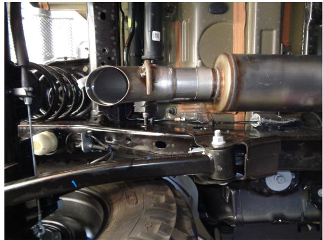
Step 4: Finish by Installing the turn down tip using the supplied clamp and fitting the hanger into the rubber insulator.
