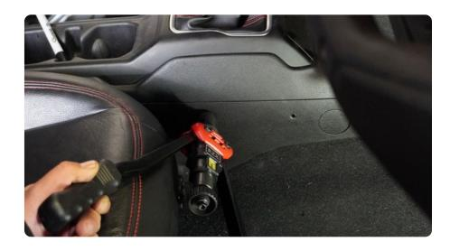
STEP 6 Use your hand to pull the panel of the center console away from the vehicle slightly, and using the provided M6 hardware and #4 allen head, install the panel until secure.
