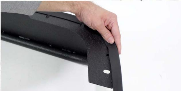
Lift your new fender flares into place. Line up the holes in the fender flare with the Jeep's OEM holes. Attach the flare with the supplied bolts, washers and nuts.
