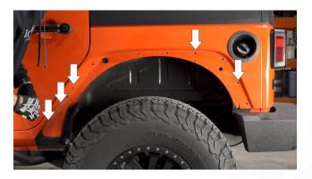
We highly recommend using a nutsert tool for installation. The thread size on the nutsert is M6-1.0. We found this tool to be helpful from MSC Direct – part #09331786
