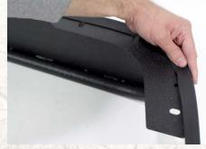
Lift your new fender flares into place. Line up the holes in the fender flare with the Jeep's OEM holes. Attach the flare with the supplied bolts, washers and nuts.
