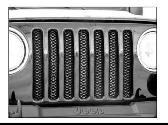
Insert rods (R16) through existing top holes and locate bottom holes for step 7.
