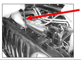
Using wide flat screwdriver, from the outside, insert through the grille and push against the rod to allow adjustment of V Brackets.
